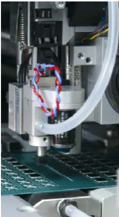
Figure 5. Rotary bond tool with hollow shaft and optical sensor (Photo courtesy of Alphasem AG)
